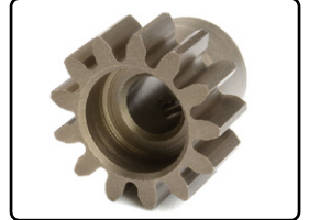
M1.0 Pinion - Hardened Steel - Shaft Diameter 5mm C-72713 • 13 Teeth (factory) C-72715 • 15 Teeth C-72717 • 17 Teeth
