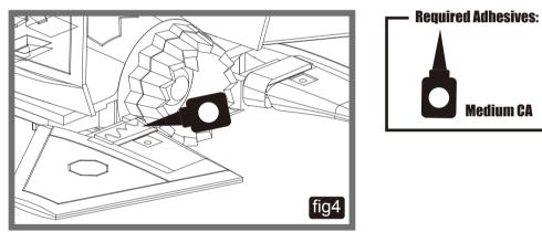
3. Install the vertical tail into place with glue. **Notce**: the vertical tail will angle towards the outboard of the plane as picture shows.
