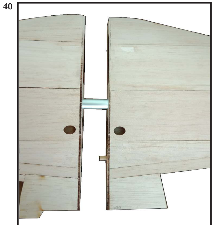
Locate and assemble the 8mm dowel at wing root for a side as (photo 38).
